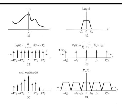
1. If  $F_s < 2f_m$ , the separate terms overlap, x(t) cannot be recovered from  $x_{\delta}(t)$ . This is called aliasing frequency
